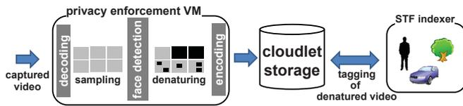
Fig. 2. GigaSight Video Processing Workflow on a Cloudlet
